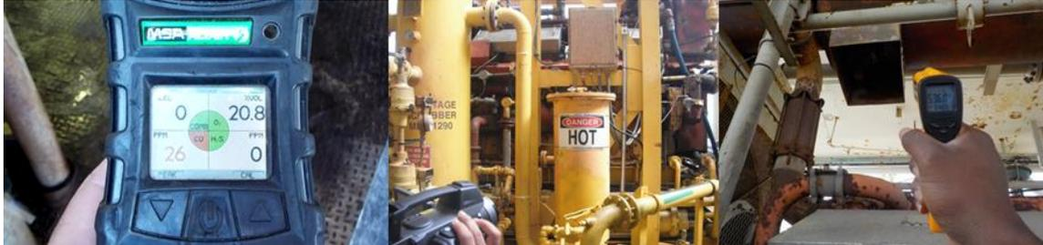
*BSEE inspectors use hand-held gas detectors, thermal cameras, and infrared thermometers during gas release risk inspections.*
