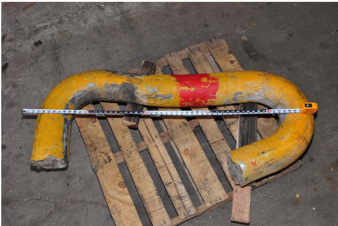
Failed Chain Link
