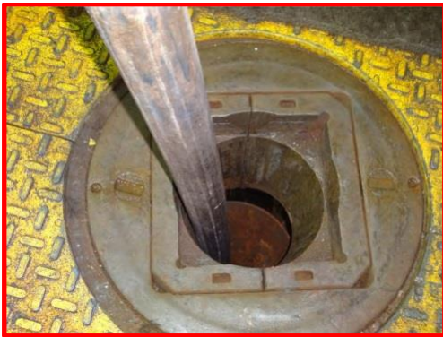
Buckled pipe leans against rotary table (left) and derrick (right) after being ejected from well
