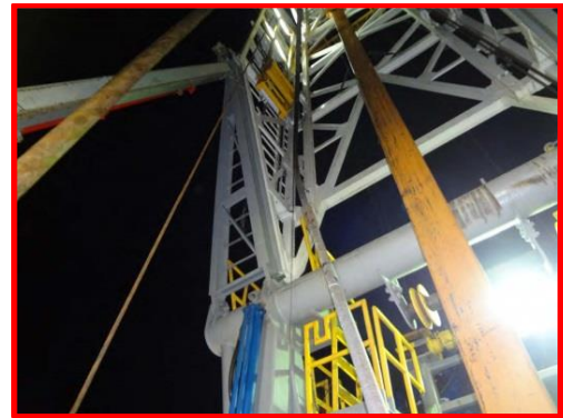
Buckled pipe leans against rotary table (left) and derrick (right) after being ejected from well
