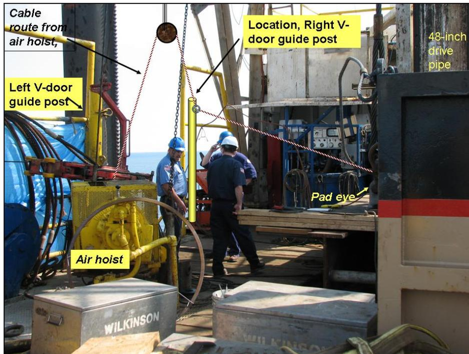
The string could not be rotated fully into position and when one of the floormen went to check the connection, the V-door guide post suddenly broke off from its weld. Propelled by the cable tension, the V-door post jumped across the floor fatally striking the floorman. A full account is available at:
