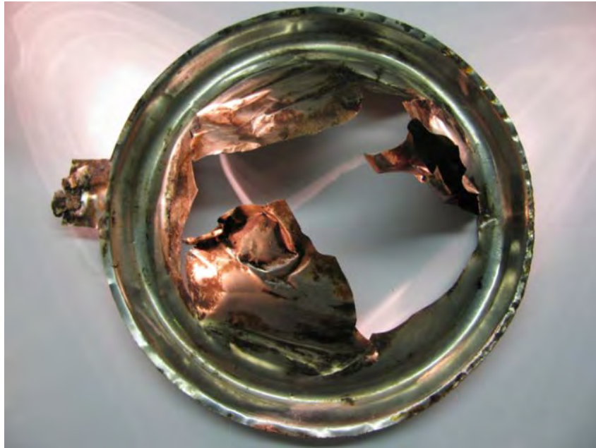
Rupture Disc Recovered from Platform's Surge Tank (BSEE Photo)
